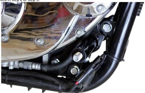
7.) Insert ½-13x3¼" (part #119-0156) through shifter side forward control mount (part #MB883XL-L). It will pass all the way through the welded spacer and threads will protrude out the other side.
